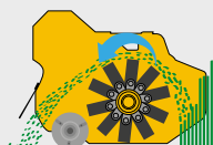
Position of the self-cleaning rear roller for discharging the mulched product behind the roller for higher output
