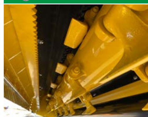
Self-cleaning roller position unloading of mulched product behind the roller for faster working speed
