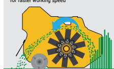
Self-cleaning roller position unloading of mulched product behind the roller for faster working speed
