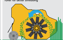
Rear roller position unloading of mulched product in front of the roller for better shredding
