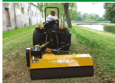
Position of the self-cleaning rear roller for discharging the mulched product behind the roller for higher output
